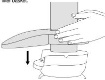
Raise the safety locking arm up and locate into the two grooves on either side of the juicer cover.
