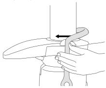
Slide the food pusher down the food chute by aligning the groove in the food pusher, with the small protrusion on the inside of the top of the feed tube.
