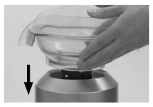
Align the arrows at the base of the stainless steel filter basket with the arrows on the motor drive coupling and push down until it clicks into place to create a secure fit with the motor base.
