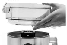
Align the arrows at the base of the Nutri Disc<sup>™</sup> with the arrows on the motor drive coupling and push down until it clicks into place. Ensure the Nutri Disc<sup>™</sup> is fitted securely inside the filter bowl surround and onto the motor base.
