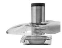
Raise the safety locking arm up and locate it into the two grooves on either side of the juicer cover. The safety locking arm should now be in a vertical position and locked into place on top of the juicer cover.
