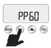
We recommend a range of between 55–65 as being optimum. Press EXIT to confirm setting and return to STANDBY mode.
