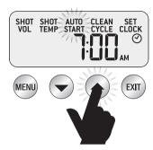
Press UP or DOWN arrow to adjust AUTO START to the desired time (default AUTO START time set at 7:00am).
