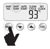
Press UP or DOWN arrow to adjust SHOT TEMP to the desired setting (range 86°C – 96°C).
