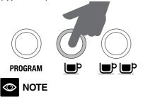
Pressing the 1 CUP or 2 CUP button during a preset shot volume will immediately stop the extraction.
